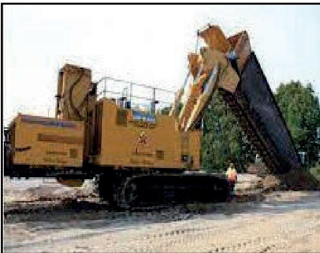
An example of the machinery that will be used for trenching
