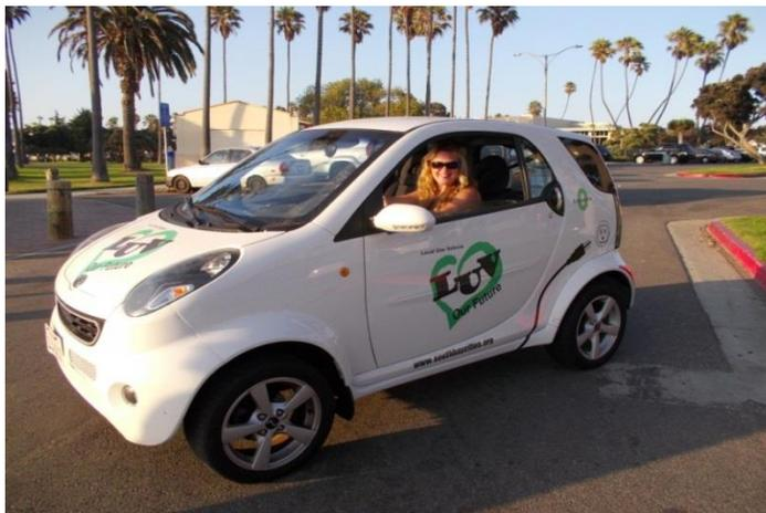
**Description:** The Wheego Whip is a compact 3 door all electric vehicle. It seats two people with a rear cargo area. The Whip features regenerative braking as well as standard “traditional” car-like features which include: am/fm radio; usb portal for an MP3 hook-up; cd player; air conditioning and heating; rear defroster; and, power locks.
