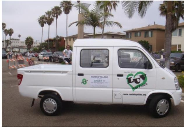
**Description:** The Vantage CrewCab is a 4 door all electric vehicle. It seats four people with front bucket seats and a back-seat bench. Additional cargo space is provided with a small cargo trunk mounted on a small rear platform. The features standard car-like features which include:
