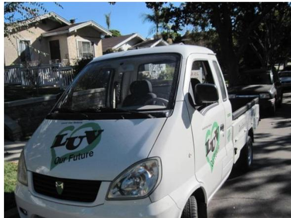
**Description:** This Miles (ZX40ST) Pick-up is a 2 door utility electric vehicle that has bench seating for 2 passengers. The model came equipped with on-board climate control (heater/air conditioner). The flat bed is approximately 6 ft. long by 4 ft. wide with “easy-hinge” side collapsible panels that fold down. This EV did not have a radio or other amenities
