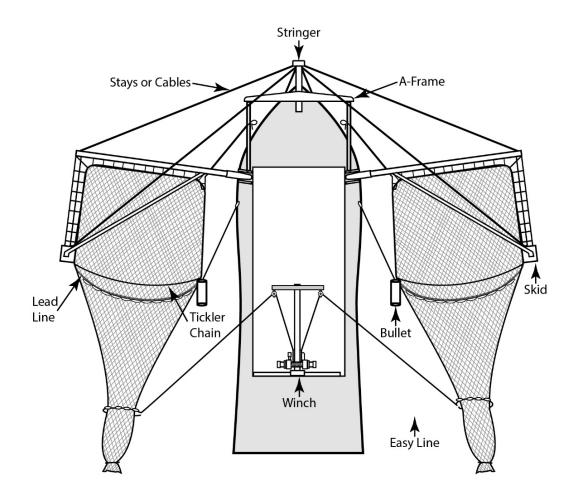
Figure 4. Schematic of skimmer trawler components.
