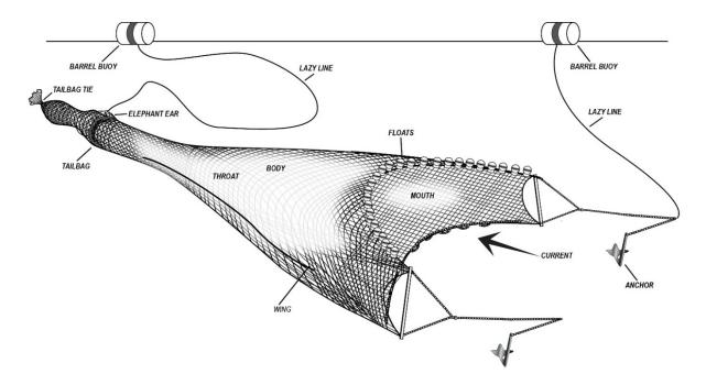
Figure 5. Schematic of channel net components.
