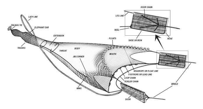
Figure 3. Schematic of otter trawl components.
