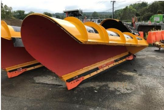
**What is it?** To combat aging equipment and the ever-rising cost of replacing plows, each year PennDOT District 1's Crawford County maintenance staff thoroughly assess plows for refurbishment or replacement. Those identified for refurbishment are disassembled, repaired, and sent to a vendor for sandblasting and refinishing.
