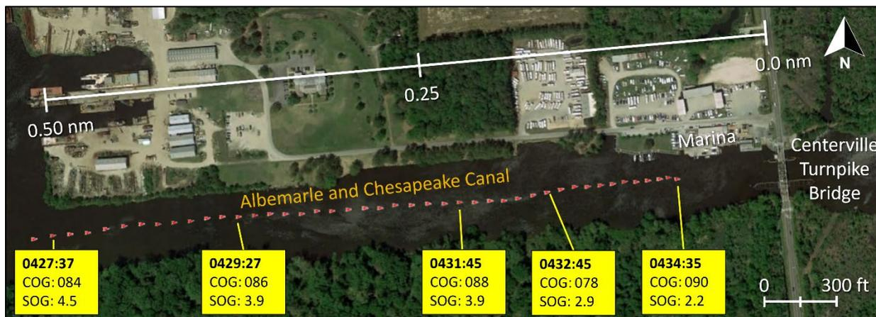
**Figure 4.** AIS track of *Island Lookout*, as represented by red arrow points. The AIS antenna was located on the towing vessel 315 feet aft of the bow of barge *BH 2903*. (Background source: Google Earth)
