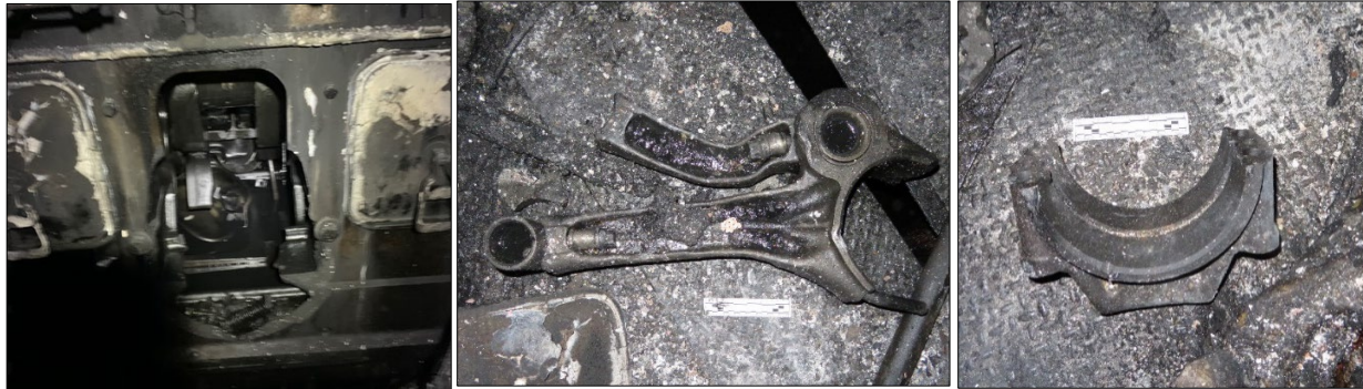
Holed crankcase at no. 4 left cylinder inspection cover ( left ), no.4 left and no. 4 right connecting rods ( middle ), and connecting rod clamp ( right ).
