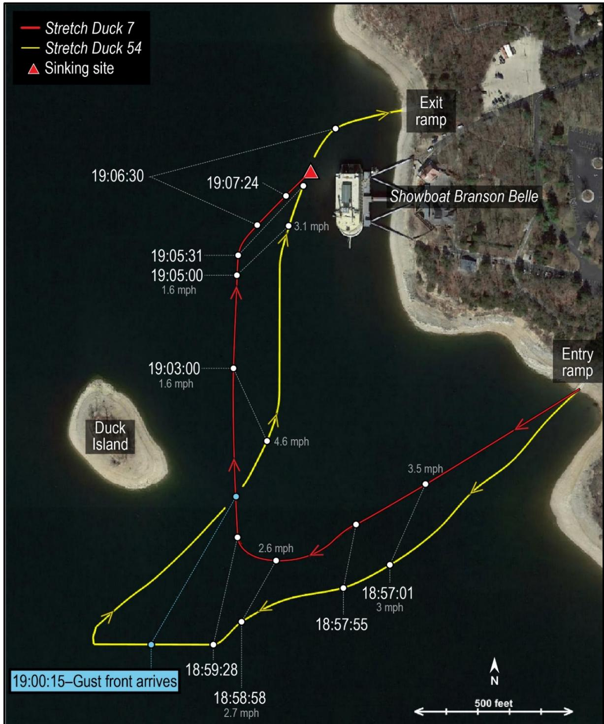
**Figure 4.** Vessel voyages on Table Rock Lake the evening of the accident. Red line represents the calculated trackline of the *Stretch Duck 7*, and yellow line represents the actual trackline of the *Stretch Duck 54* based on GPS data.<sup>13</sup>
