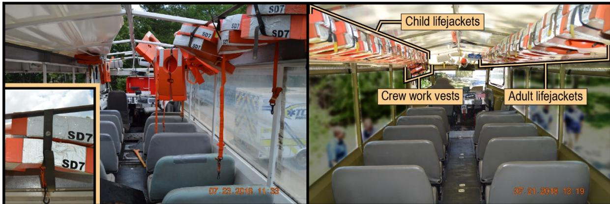
**Figure 13.** Lifejackets recovered on the *Stretch Duck 7* (left) compared to how they would have been stowed, as shown on the similar vessel *Stretch Duck 9* (right). Infant lifejackets would have been stowed aft of the child lifejackets. (Source: Missouri State Highway Patrol)
