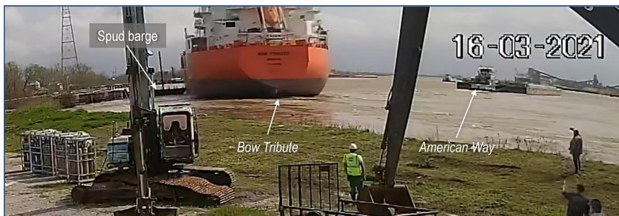
**Figure 5.** CCTV footage looking downriver at 1522:26 shows the *Bow Tribute* when it struck the spud barge protecting the New River water intake pipes. (Source: Crosby Dredging)
