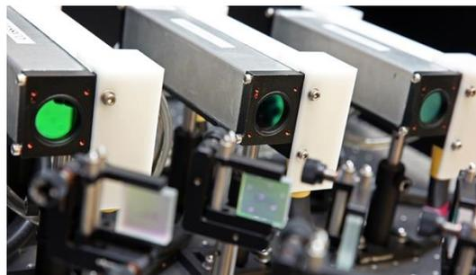
Diode-based Additive Manufacturing (DiAM) uses high-powered arrays of laser diodes and a specialized laser modulator developed for the National Ignition Facility (NIF) to flash print an entire layer of metal powder at once.
