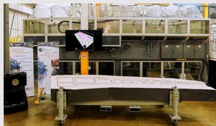
In 2016, ORNL's BAAM printed the world's largest solid 3D-printed object: a trim-and-drill tool for Boeing.
