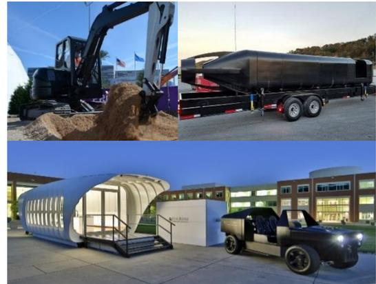
Images (clockwise from top-left): fully-functional AM-fabricated excavator; 3D-printed submarine; and AM-developed home and natural gas vehicle.
