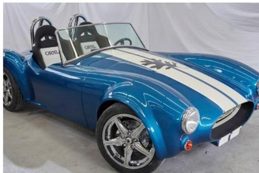
Using carbon fiber-enhanced polymers, the BAAM printer produced the frame and body of a full-scale Shelby Cobra in 2014; body panels feature a surface variation of 0.020 inches.
