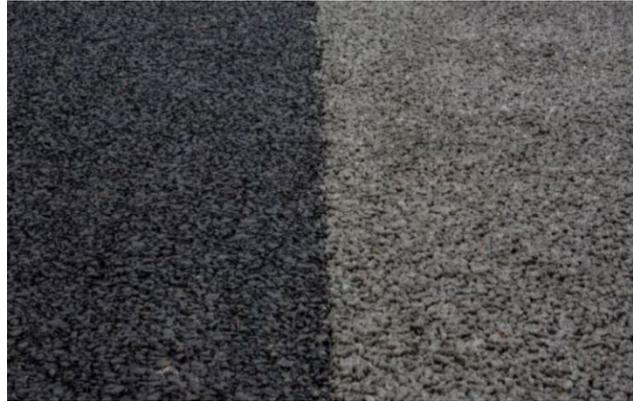
POROUS ASPHALT AND PERVIOUS CONCRETE
