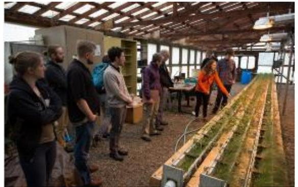
MEMBERS OF THE PUGET SOUND STORMWATER SCIENCE TEAM TESTING A GREEN STORMWATER TECHNOLOGY: COMPOST-AMENDED BIOSWALES.
