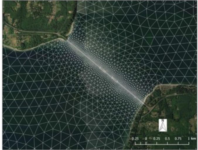
SALISH SEA MODEL GRID WITH REFINEMENT NEAR THE HOOD CANAL BRIDGE REGION TO FACILITATE INCORPORATION OF THE BRIDGE BLOCK IN THE SIMULATION.
