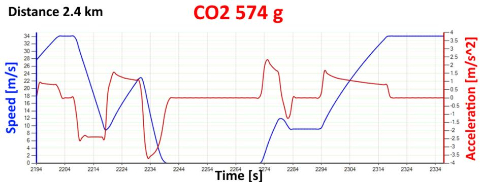
Figure 8: Single vehicle speed profile, with accident
