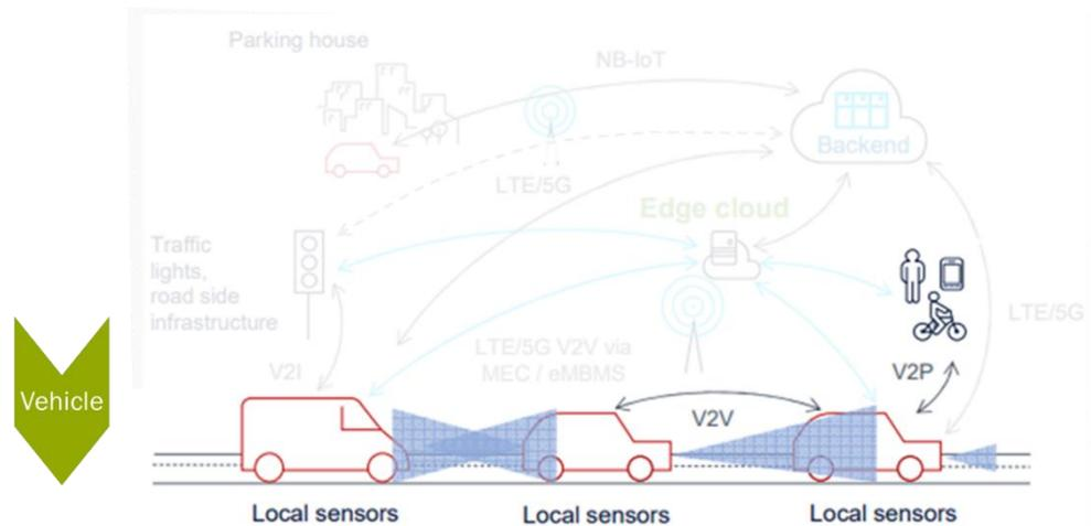
Figure 13: Implementation options with V2V communication.
