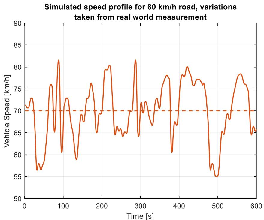
Figure 12: Simulated speed profile for an 80 km/h road, variations taken from real world measurement.
