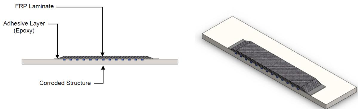
**(a): Repair System – Corroded Structure, Adhesive Layer (Epoxy), FRP Laminate**
