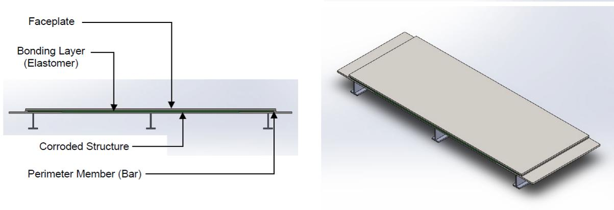
**(c): Repair System – Corroded Structure, Perimeter Member (Bar), Bonding Layer (Elastomer) and Faceplate**
