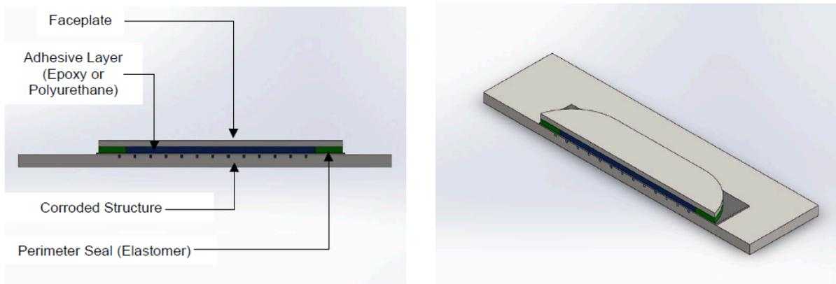
**(b): Repair System – Corroded Structure, Perimeter Seal (Elastomer), Adhesive Layer (Epoxy or Polyurethane) and Faceplate**
